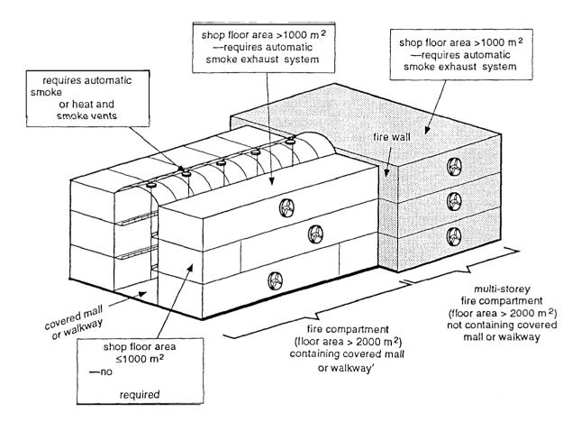
FIGURE 7.3 SPRINKLERED THREE STOREY BUILDING
