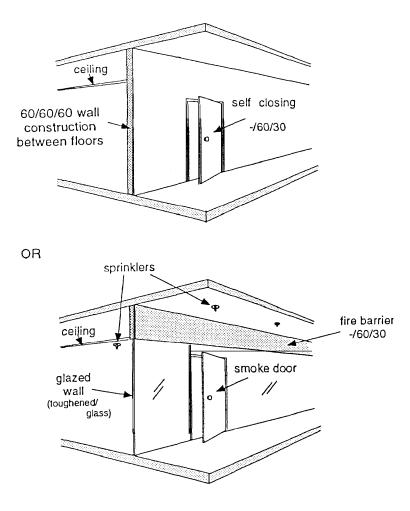
FIGURE 8.2 BOUNDING WALL CONSTRUCTION
