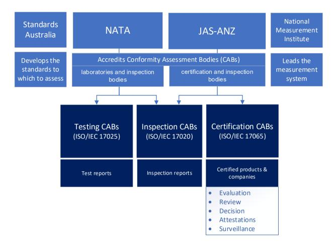
Figure 4: Key elements of Australia's Quality Conformance Infrastructure
