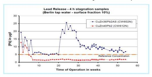
Figure 2: Effects of dezincification on lead releasing from the bulk alloy<sup>22</sup>
