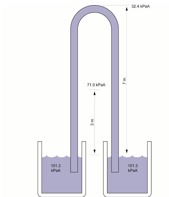
Figure C.5 Pressure relationships in a continuous fluid system at the same elevation
