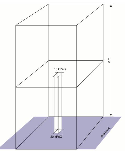
If this process was repeated with a third cubic metre of water, the pressures at the base of each cube would be 30 kPaG, 20 kPaG, and 10 kPaG, respectively. It is evident that pressure varies with depth below a free water surface. In general, each metre of elevation change within a liquid, changes the pressure by an amount equal to the weight-per-unit area of 1 metre of the liquid. The rate of increase for water is 10 kPaG per metre of depth.
