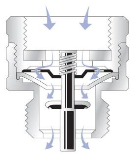
When the water supply is turned off, the device vents to atmosphere, therefore protecting against backsiphonage conditions. Typical installation is shown in Figure 6.6.
