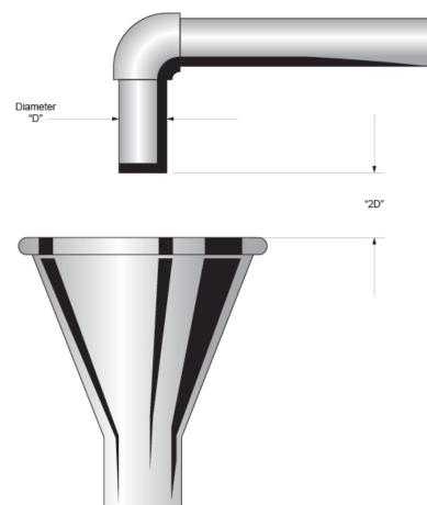
An AG can cause a corresponding loss of pressure to downstream outlets. However, they are an extremely effective backflow preventer when used to prevent backsiphonage and backpressure conditions. Consequently, AGs are primarily used at end of line services where reservoirs or storage tanks are desired.
